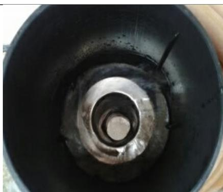
*Water moving in a spiral motion on the inner surface of the cylindrical mesh*
