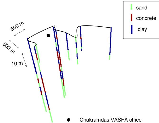
**Figure 6. Collected well logs in and around Chakramdas village**
