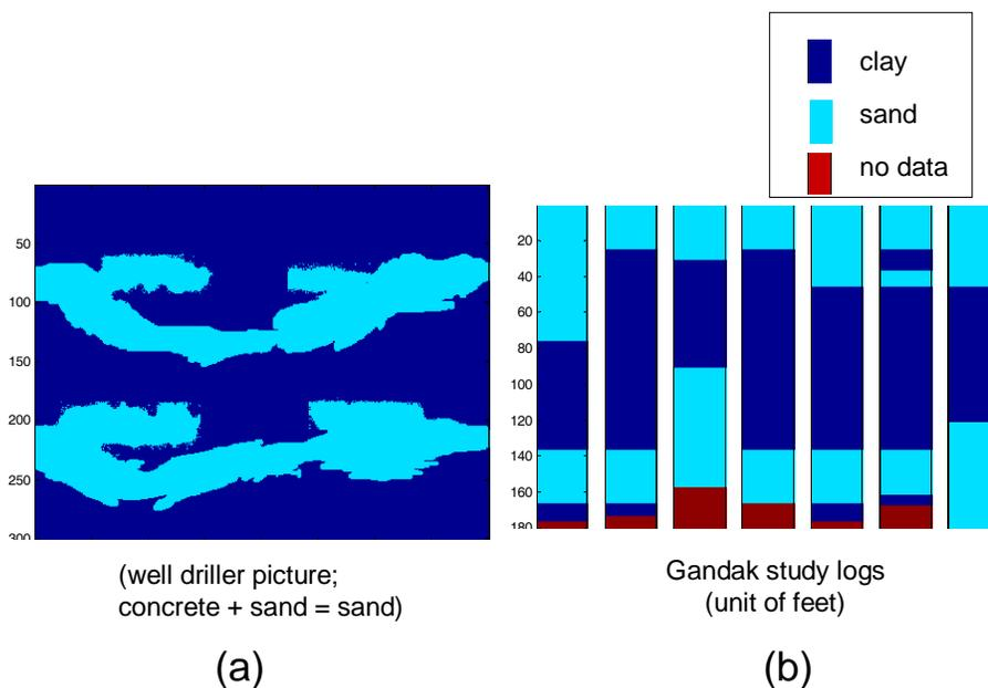
**Figure 5. Comparison of conceptual image (a) with logs provided in the Gandak report (b) (NIH, 2000)**
