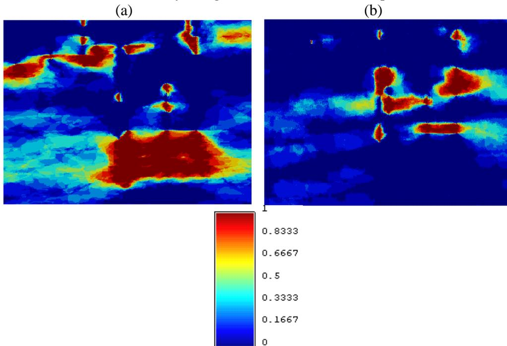
Figure 10. Probability of occurrence of sand (a) and concrete (b) based on averaging of 15 equally likely depictions
