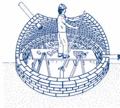
Making the brick dome
