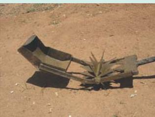
The weeders that are available in the market are a bit costly. There are some problems with the design also. When these are being used in heavy soils, there are several problems. Different weeders were studied and by combining the advantages of each one, a new 'mandava' weeder has been designed. The weeder got its name after 'Chinna Mandava', a village in Khammam district in Andhra Pradesh, where it has been tested and fine tuned.
