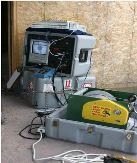
Fig- 4, Bore Hole video camera.
